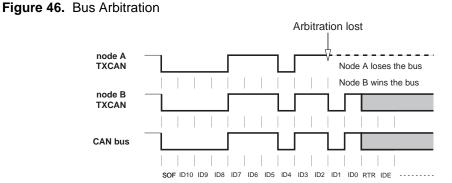
The CAN protocol handles bus accesses according to the concept called "Carrier Sense Multiple Access with Arbitration on Message Priority".
