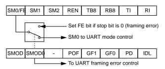
When this feature is enabled, the receiver checks each incoming data frame for a valid stop bit. An invalid stop bit may result from noise on the serial lines or from simultaneous transmission by two CPUs. If a valid stop bit is not found, the Framing Error bit (FE) in SCON register bit is set.
