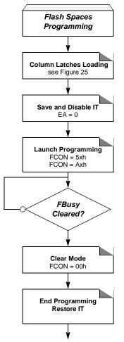
Figure 26. Flash and Extra Row Programming Procedure
