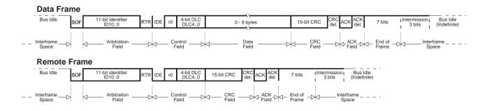
A message in the CAN standard frame format begins with the "Start Of Frame (SOF)", this is followed by the "Arbitration field" which consist of the identifier and the "Remote Transmission Request (RTR)" bit used to distinguish between the data frame and the data request frame called remote frame. The following "Control field" contains the "IDentifier Extension (IDE)" bit and the "Data Length Code (DLC)" used to indicate the
