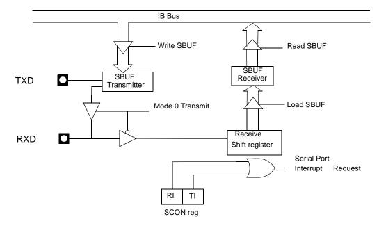
**Framing Error Detection** Framing bit error detection is provided for the three asynchronous modes. To enable the framing bit error detection feature, set SMOD0 bit in PCON register.
