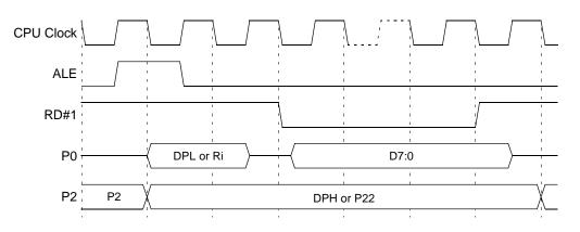
Notes: 1. RD# signal may be stretched using M0 bit in AUXR register.2. When executing MOVX @Ri instruction, P2 outputs SFR content.
