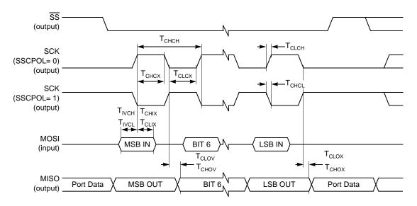
Figure 86. SPI Master Waveforms (SSCPHA= 0)
