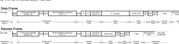
Figure 44. CAN Extended Frames
