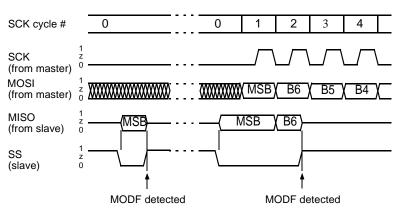
Note: when SS is discarded (SS disabled) it is not possible to detect a MODF error in slave mode because the SPI is internally selected. Also the SS pin becomes a general purpose I/O.
