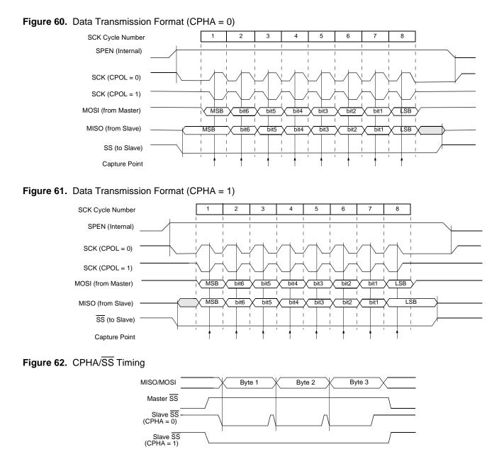
As shown in Figure 60, the first SCK edge is the MSB capture strobe. Therefore, the Slave must begin driving its data before the first SCK edge, and a falling edge on the  $\overline{SS}$  pin is used to start the transmission. The  $\overline{SS}$  pin must be toggled high and then low between each Byte transmitted (Figure 62).
