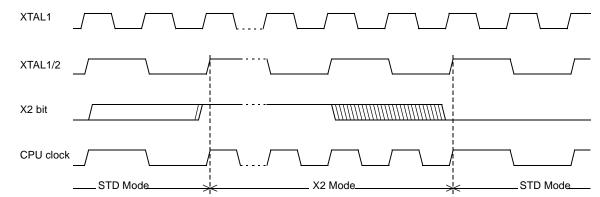
Figure 6. Mode Switching Waveforms
