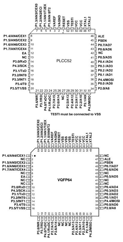
**TESTI** must be connected to VSS
