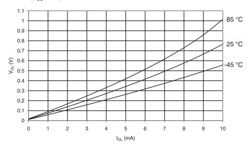
Figure 30-29. ATmega169A. I/O Pin Output Voltage vs. Sink Current, Ports A, C, D, E, F, G  $(V_{CC} = 2.7V)$
