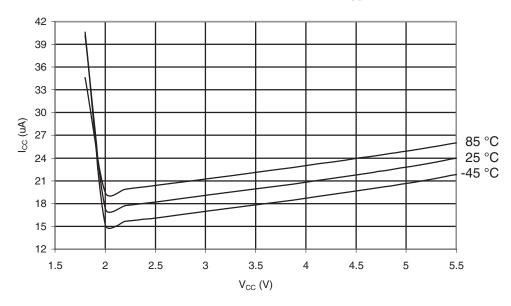
Figure 30-599.ATmega6490P: Active Supply Current with ADC at 50kHz vs. V<sub>CC</sub>
