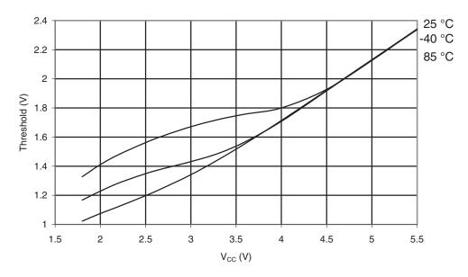
Figure 30-282.ATmega3290A: Reset Input Threshold Voltage vs. V<sub>CC</sub> (V<sub>IL</sub>,Reset Pin Read as "0")
