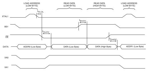
Note: 1. The timing requirements shown in Figure 28-7 on page 323 (i.e., t<sub>DVXH</sub>, t<sub>XHXL</sub>, and t<sub>XLDX</sub>) also apply to reading operation.
