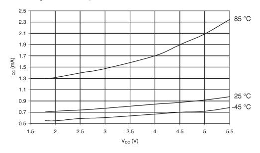
**Figure 30-502.** ATmega6490A: Standby Supply Current vs.  $V_{CC}$  (Xtall and Resonator, Watchdog Timer Disabled)
