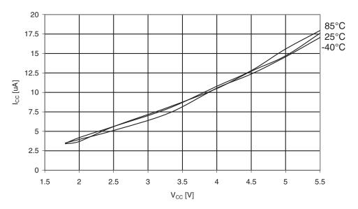
Figure 30-360.ATmega3290PA: Analog Comparator Current vs. V<sub>CC</sub>
