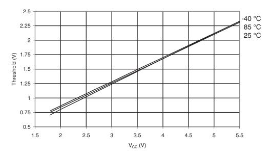
Figure 30-223. ATmega329 PA: Reset Input Pin Hysteresis vs.  $V_{\rm CC}$
