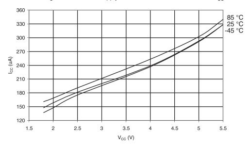
Figure 30-601.ATmega6490P: Active Supply Current with ADC at 1MHz vs. V<sub>CC</sub>
