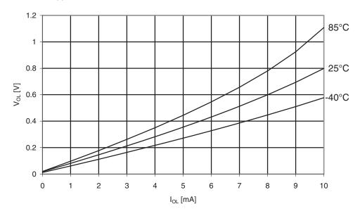
Figure 30-214. ATmega329 PA: I/O Pin Output Voltage vs. Sink Current, Ports A, C, D, E, F, G  $(V_{CC} = 1.8V)$
