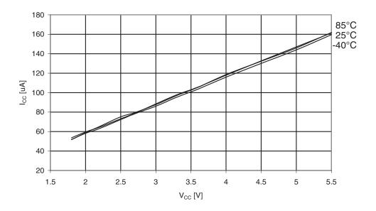
Figure 30-299.ATmega3290A: Watchdog Timer Current vs. V<sub>CC</sub>
