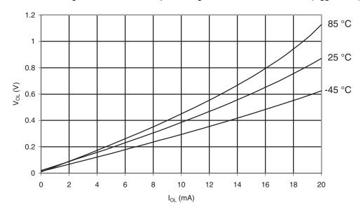
Figure 30-581. ATmega6490P: I/O Pin Output Voltage vs. Sink Current, Port B ( $V_{CC} = 1.8V$ )
