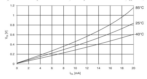
Figure 30-217.ATmega329PA: I/O Pin Output Voltage vs. Sink Current, Port B (V<sub>CC</sub> = 1.8V)
