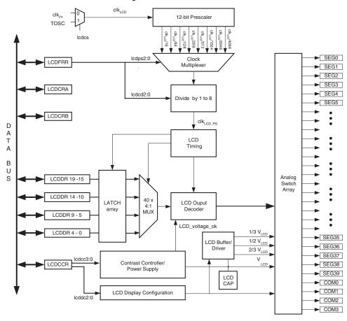
Figure 24-1. LCD Module Block Diagram
