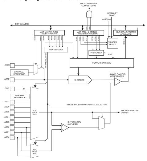
Figure 23-1. Analog to Digital Converter Block Schematic
