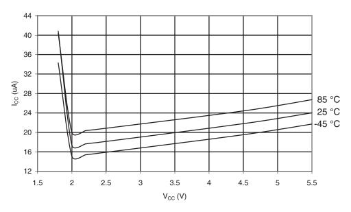
Figure 30-115.ATmega169PA: Active Supply Current with ADC at 50kHz vs. V<sub>CC</sub>
