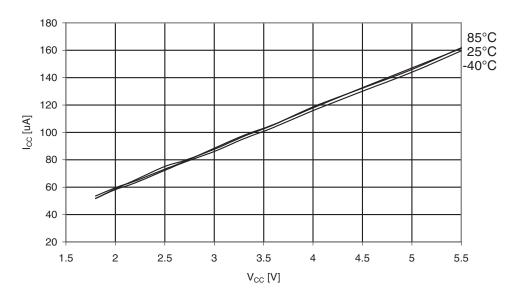
Figure 30-179.ATmega329A: Watchdog Timer Current vs. V<sub>CC</sub>
