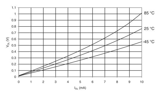
Figure 30-91. ATmega169PA. I/O Pin Output Voltage vs. Sink Current, Ports A, C, D, E, F, G  $(V_{CC}=2.7V)$
