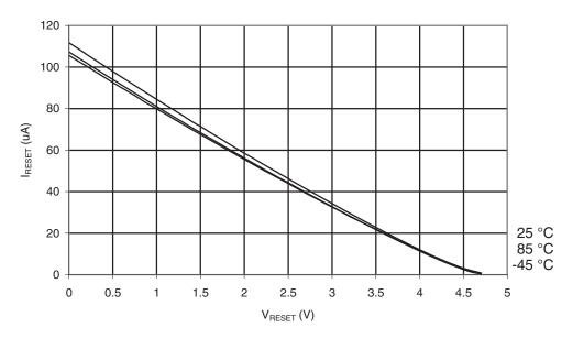
Figure 30-20. ATmega169A: Reset Pull-up Resistor Current vs. Reset Pin Voltage (V<sub>CC</sub> = 2.7V)
