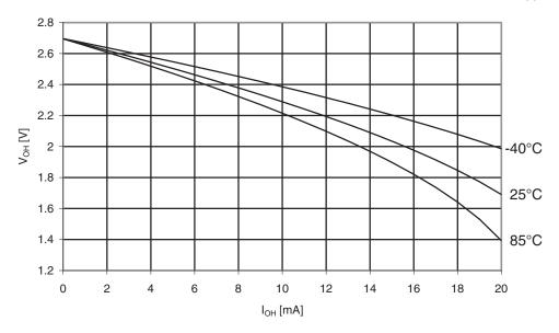
Figure 30-331. ATmega3290 PA: I/O Pin Output Voltage vs. Source Current, Port B ( $V_{CC} = 1.8V$ )
