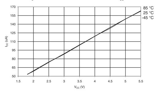
Figure 30-420.ATmega649A: Watchdog Timer Current vs. V<sub>CC</sub>
