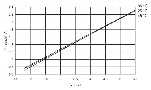
Figure 30-526. ATmega6490A: Reset Input Pin Hysteresis vs.  $V_{\rm CC}$
