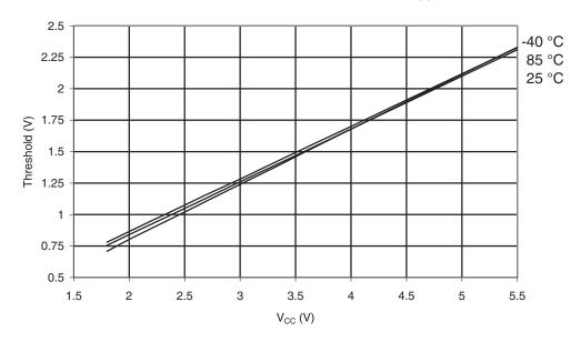
Figure 30-163. ATmega329A: Reset Pin Input Hysteresis vs.  $V_{CC}$
