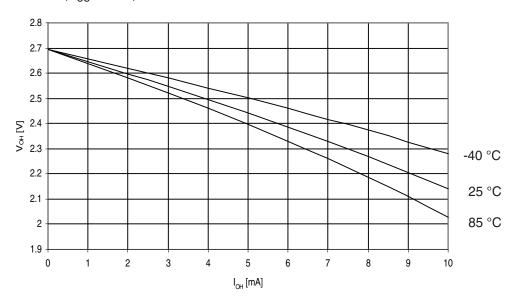
Figure 30-148. ATmega329A: I/O Pin Output Voltage vs. Source Current, Ports A, C, D, E, F, G  $(V_{CC} = 1.8V)$
