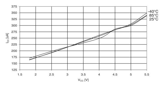
Figure 30-178. ATmega329A: AREF External Reference Current vs. V<sub>CC</sub>
