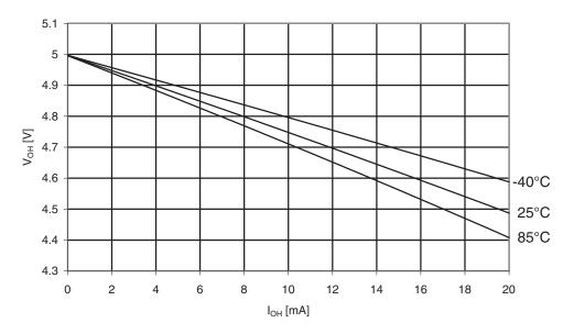
Figure 30-150.ATmega329A: I/O Pin Output Voltage vs. Source Current, Port B (V<sub>CC</sub> = 2.7V)
