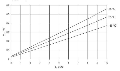
**Figure 30-455.** ATmega649P. I/O Pin Output Voltage vs. Sink Current, Ports A, C, D, E, F, G  $(V_{CC}=2.7V)$
