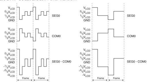
Figure 24-7. Default and Low Power Waveform
