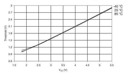
Figure 30-219.ATmega329PA. I/O Pin Input Threshold Voltage vs. V<sub>CC</sub> (V<sub>IL</sub>, I/O Pin Read as "0")
