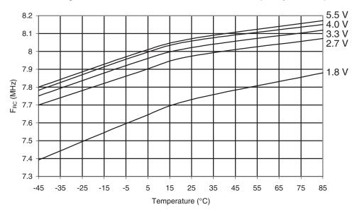
Figure 30-535.ATmega6490A: Calibrated 8MHz RC Oscillator Frequency vs. V<sub>CC</sub>
