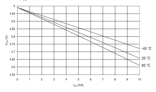
**Figure 30-510.** ATmega6490A: I/O Pin Output Voltage vs. Source Current, Ports A, C, D, E, F, G  $(V_{CC}=2.7V)$
