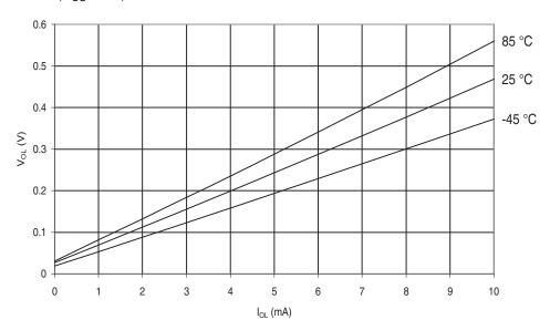
**Figure 30-516.**ATmega6490A. I/O Pin Output Voltage vs. Sink Current, Ports A, C, D, E, F, G  $(V_{CC} = 2.7V)$
