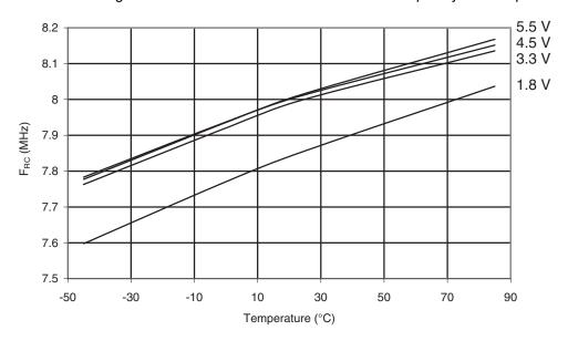
Figure 30-112. ATmega169PA: Calibrated 8MHz RC Oscillator Frequency vs.  $V_{CC}$
