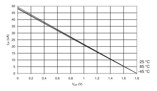
Figure 30-81. ATmega169PA: Reset Pull-up Resistor Current vs. Reset Pin Voltage (V<sub>CC</sub> = 5V)
