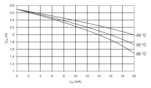
Figure 30-27. ATmega169A: I/O Pin Output Voltage vs. Source Current, Port B (V<sub>CC</sub> = 1.8V)
