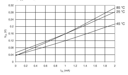
Figure 30-518.ATmega6490A: I/O Pin Output Voltage vs. Sink Current, Port B (V<sub>CC</sub> = 5V)
