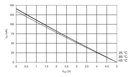
Figure 30-17. ATmega169A: I/O Pin Pull-up Resistor Current vs. Input Voltage (V<sub>CC</sub> = 2.7V)
