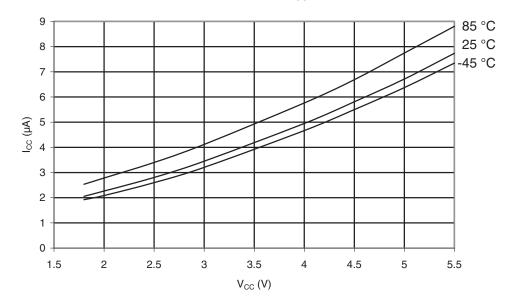
Figure 30-10. ATmega169A: Idle Supply Current vs. V<sub>CC</sub> (32kHz Watch Crystal)
