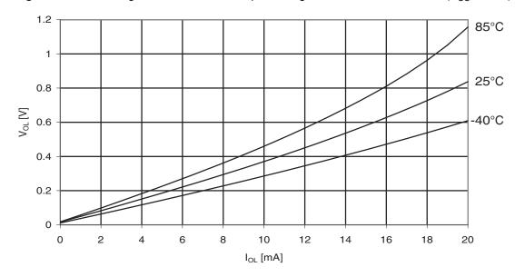
Figure 30-337.ATmega3290PA: I/O Pin Output Voltage vs. Sink Current, Port B (V<sub>CC</sub> = 1.8V)
