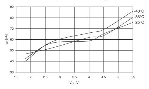
Figure 30-241.ATmega329PA: Programming Current vs. V<sub>CC</sub>
