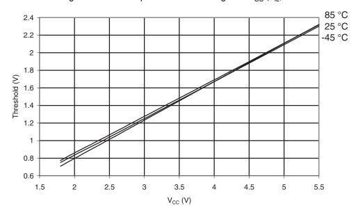
Figure 30-404.ATmega649A: Reset Input Pin Hysteresis vs. V<sub>CC</sub>
