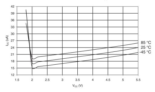
Figure 30-416.ATmega649A: Active Supply Current with ADC at 50kHz vs. V<sub>CC</sub>
