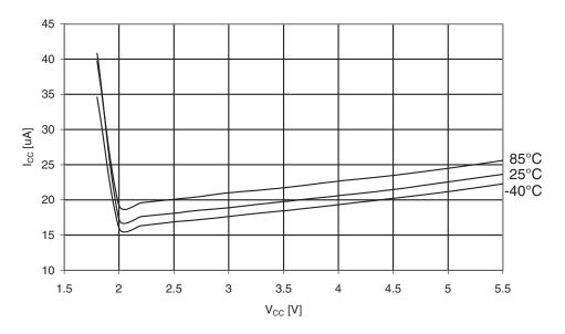
Figure 30-175.ATmega329A: Active Supply Current with ADC at 50kHz vs. V<sub>CC</sub>
