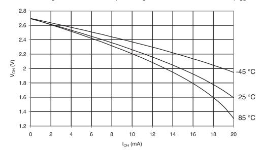
Figure 30-575. ATmega6490P: I/O Pin Output Voltage vs. Source Current, Port B ( $V_{CC} = 1.8V$ )
