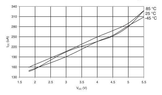
Figure 30-541.ATmega6490A: AREF External Reference Current vs. V<sub>CC</sub>
