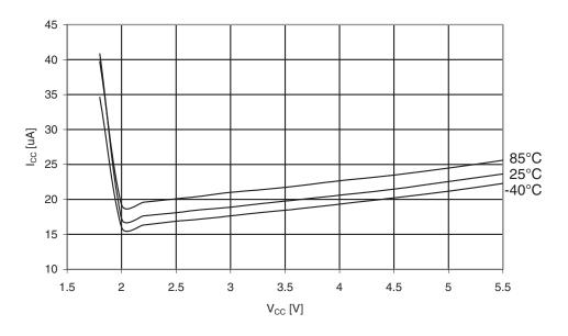
Figure 30-295.ATmega3290A: Active Supply Current with ADC at 50kHz vs. V<sub>CC</sub>
