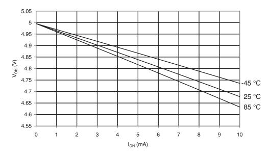
**Figure 30-23.** ATmega169A: I/O Pin Output Voltage vs. Source Current, Ports A, C, D, E, F, G  $(V_{CC} = 2.7V)$
