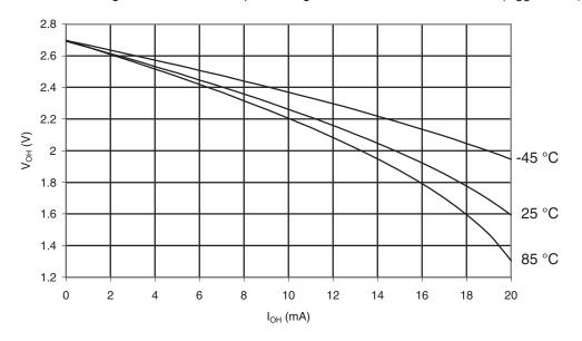
Figure 30-453. ATmega649P: I/O Pin Output Voltage vs. Source Current, Port B ( $V_{CC} = 1.8V$ )
