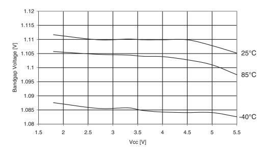
Figure 30-288. ATmega3290A: Bandgap Voltage vs. Temperature
