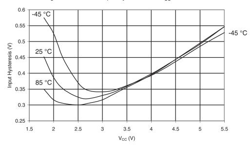
Figure 30-585.ATmega6490P: Reset Input Threshold Voltage vs. V<sub>CC</sub> (V<sub>IH</sub>,Reset Pin Read as "1")
