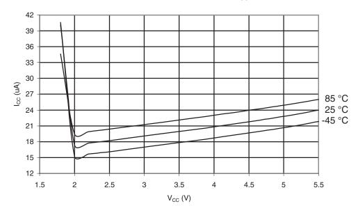
Figure 30-477.ATmega649P: Active Supply Current with ADC at 50kHz vs. V<sub>CC</sub>
