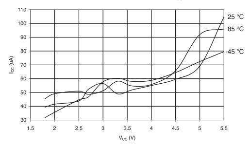
Figure 30-544.ATmega6490A: Programming Current vs. V<sub>CC</sub>
