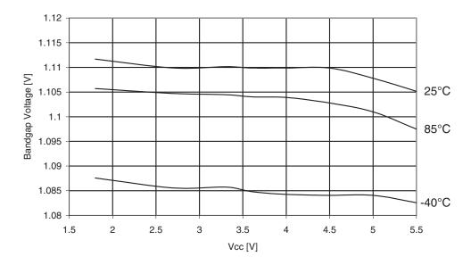
Figure 30-228. ATmega329PA: Bandgap Voltage vs. Temperature
