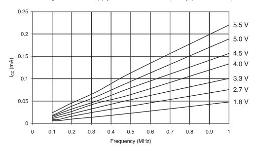
Figure 30-7. ATmega169A: Idle Supply Current vs. Frequency (1 - 16MHz)
