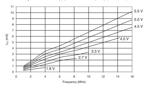
Figure 30-3. ATmega169A: Active Supply Current vs. V<sub>CC</sub> (Internal RC Oscillator, 8MHz)
