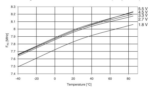
Figure 30-292. ATmega3290A: Calibrated 8MHz RC Oscillator Frequency vs.  $V_{CC}$
