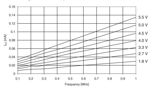
**Figure 30-303.**ATmega3290A: Reset Supply Current vs. V<sub>CC</sub> (1 - 20MHz, Excluding Current Through The Reset Pull-up)
