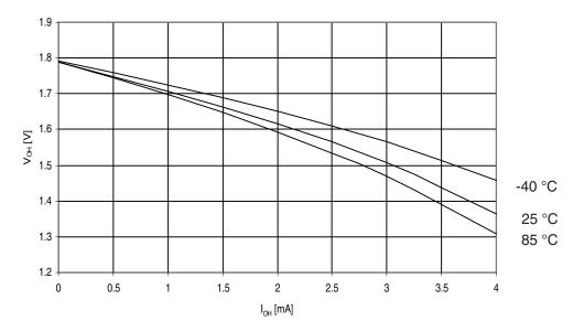
Figure 30-149.ATmega329A: I/O Pin Output Voltage vs. Source Current, Port B (V<sub>CC</sub>= 5V)
