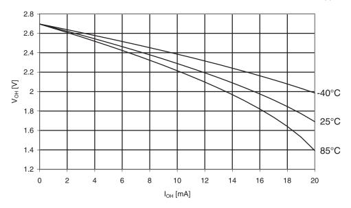
Figure 30-271. ATmega3290A: I/O Pin Output Voltage vs. Source Current, Port B (V<sub>CC</sub> = 1.8V)
