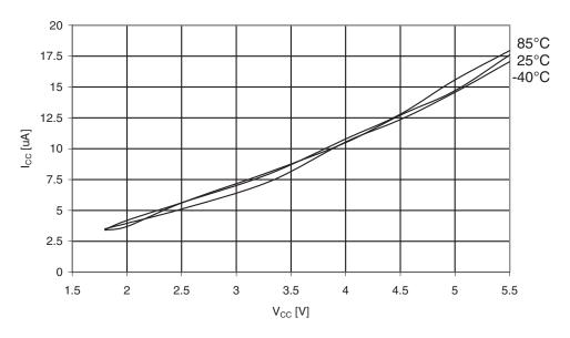
Figure 30-240.ATmega329PA: Analog Comparator Current vs. V<sub>CC</sub>
