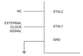
When this clock source is selected, start-up times are determined by the SUT Fuses as shown in Table 9-13.
