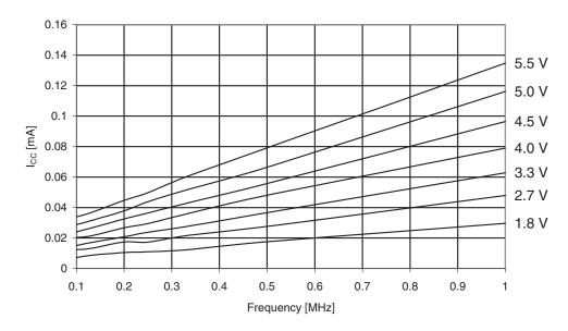
**Figure 30-183.**ATmega329A: Reset Supply Current vs. V<sub>CC</sub> (1 - 20MHz, Excluding Current Through The Reset Pull-up)
