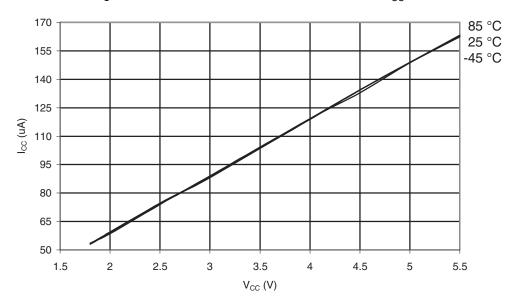
Figure 30-481.ATmega649P: Watchdog Timer Current vs. V<sub>CC</sub>
