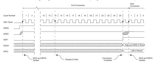
Figure 23-5. ADC Timing Diagram, Single Conversion
