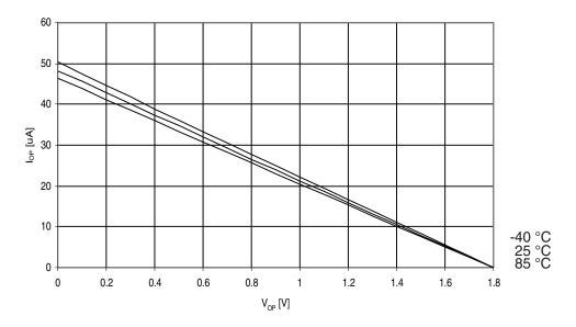
Figure 30-143. ATmega329A: Reset Pull-up Resistor Current vs. Reset Pin Voltage ( $V_{CC} = 5V$ )
