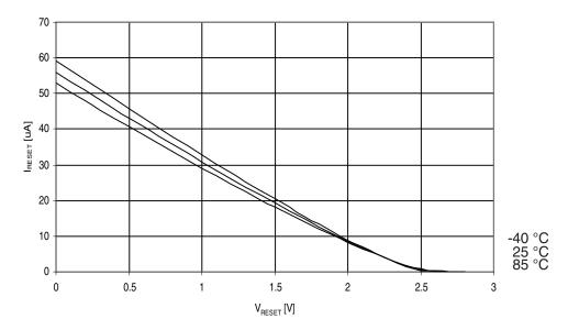
Figure 30-145. ATmega329A: Reset Pull-up Resistor Current vs. Reset Pin Voltage (V<sub>CC</sub> = 1.8V)
