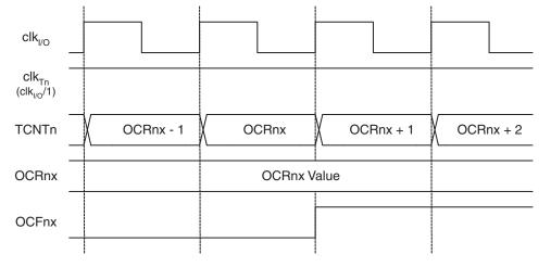
Figure 16-11 shows the same timing data, but with the prescaler enabled.
