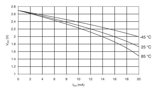
Figure 30-89. ATmega169PA: I/O Pin Output Voltage vs. Source Current, Port B (V<sub>CC</sub> = 1.8V)
