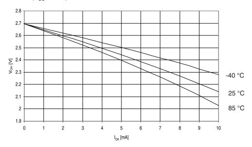
Figure 30-268. ATmega3290 A: I/O Pin Output Voltage vs. Source Current, Ports A, C, D, E, F, G  $(V_{CC}=1.8V)$
