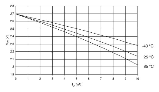
Figure 30-328. ATmega3290 PA: I/O Pin Output Voltage vs. Source Current, Ports A, C, D, E, F, G ( $V_{CC} = 1.8V$ )
