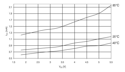
The differential current consumption between Power-save with WD disabled and 32kHz TOSC represents the current drawn by Timer/Counter2.
