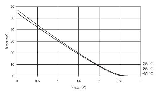
Figure 30-83. ATmega169PA: Reset Pull-up Resistor Current vs. Reset Pin Voltage (V<sub>CC</sub>=1.8V)
