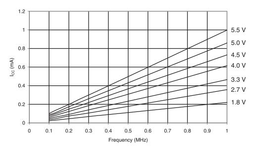
Figure 30-64. ATmega169PA: Active Supply Current vs. Frequency (1 - 16MHz)
