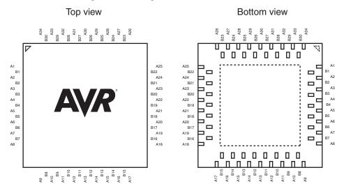
Table 1-1. DRQFN-64 Pinout ATmega169A/ATmega169PA
