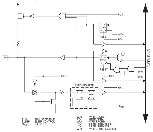
WRx, WPx, WDx, RRx, RPx, and RDx are common to all pins within the same port. clk<sub>I/O</sub>, SLEEP, and PUD are common to all ports.
