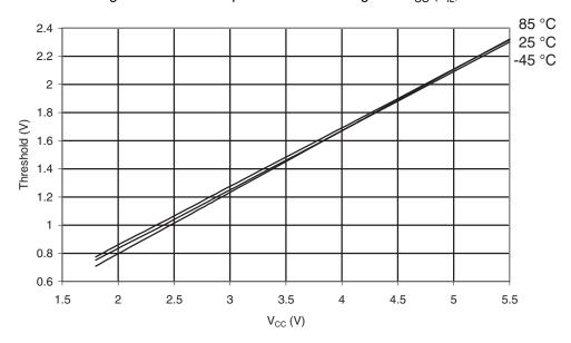
Figure 30-587.ATmega6490P: Reset Input Pin Hysteresis vs.  $V_{CC}$
