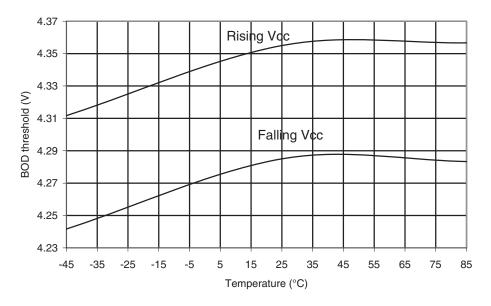
Figure 30-41. ATmega169A: BOD Thresholds vs. Temperature (BOD Level is 2.7V)
