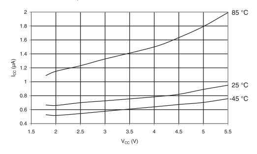
**Figure 30-15.** ATmega169A: Standby Supply Current vs.  $V_{CC}$  (Xtall and Resonator, Watchdog Timer Disabled)
