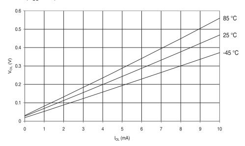
**Figure 30-394.** ATmega649A. I/O Pin Output Voltage vs. Sink Current, Ports A, C, D, E, F, G  $(V_{CC} = 2.7V)$
