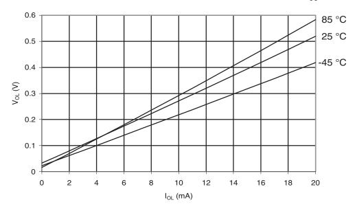
Figure 30-397. ATmega649A: I/O Pin Output Voltage vs. Sink Current, Port B ( $V_{CC} = 2.7V$ )
