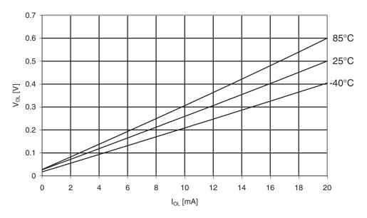
Figure 30-216. ATmega329PA: I/O Pin Output Voltage vs. Sink Current, Port B ( $V_{CC} = 2.7V$ )
