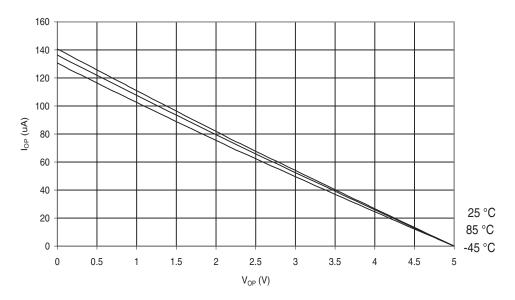
Figure 30-504.ATmega6490A: I/O Pin Pull-up Resistor Current vs. Input Voltage (V<sub>CC</sub> = 2.7V)
