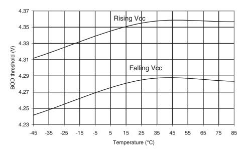
Figure 30-103. ATmega169PA: BOD Thresholds vs. Temperature (BOD Level is 2.7V)
