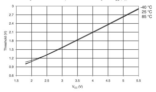
Figure 30-279.ATmega3290A: I/O Pin Input Threshold Voltage vs. V<sub>CC</sub> (V<sub>IL</sub>, I/O Pin Read as "0")
