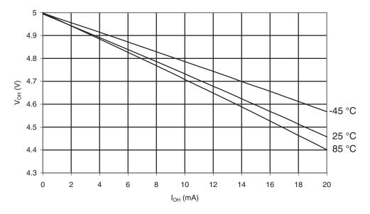
Figure 30-574. ATmega6490P: I/O Pin Output Voltage vs. Source Current, Port B ( $V_{CC} = 2.7V$ )
