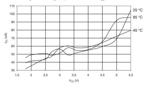
Figure 30-422.ATmega649A: Programming Current vs. V<sub>CC</sub>
