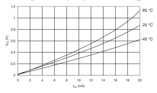
Figure 30-459. ATmega649P: I/O Pin Output Voltage vs. Sink Current, Port B ( $V_{CC} = 1.8V$ )
