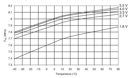
Figure 30-413. ATmega649A: Calibrated 8MHz RC Oscillator Frequency vs. V<sub>CC</sub>
