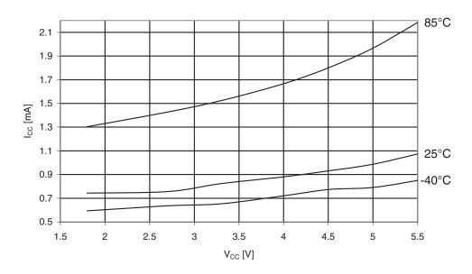
Figure 30-199. ATmega329PA Standby Supply Current vs.  $V_{CC}$  (Xtall and Resonator, Watchdog Timer Disabled)
