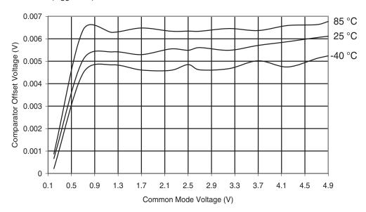
Figure 30-108. ATmega 169 PA: Analog Comparator Offset Voltage vs. Common Mode Voltage  $(V_{CC}=2.7V)$
