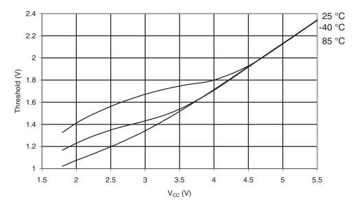
Figure 30-222. ATmega329PA: Reset Input Threshold Voltage vs. V<sub>CC</sub> (V<sub>IL</sub>,Reset Pin Read as "0")
