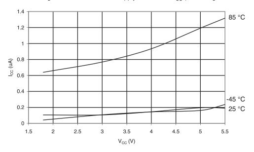
Figure 30-74. ATmega169PA: Power-down Supply Current vs. V<sub>CC</sub> (Watchdog Timer Enabled)
