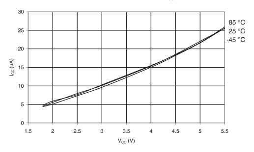
Figure 30-120.ATmega169PA: Analog Comparator Current vs. V<sub>CC</sub>
