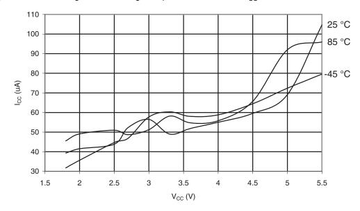
Figure 30-483.ATmega649P: Programming Current vs. V<sub>CC</sub>
