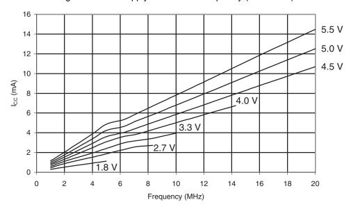
Figure 30-372. ATmega649A: Idle Supply Current vs.  $V_{CC}$  (Internal RC Oscillator, 8MHz)
