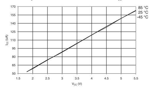
Figure 30-603.ATmega6490P: Watchdog Timer Current vs. V<sub>CC</sub>
