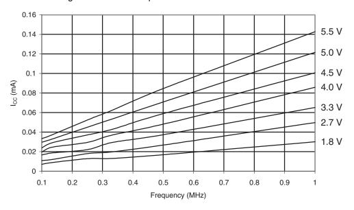
**Figure 30-546.**ATmega6490A: Reset Supply Current vs. V<sub>CC</sub> (1 - 20MHz, Excluding Current Through The Reset Pull-up)
