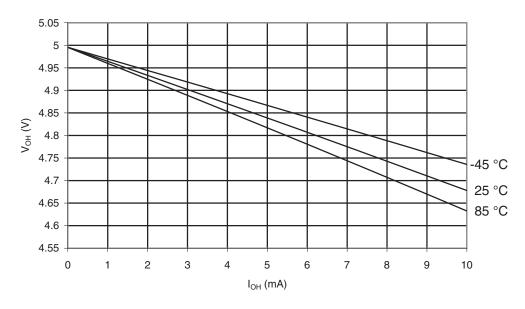
**Figure 30-85.** ATmega169PA: I/O Pin Output Voltage vs. Source Current, Ports A, C, D, E, F, G  $(V_{CC} = 2.7V)$
