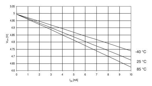
**Figure 30-147.** ATmega329A: I/O Pin Output Voltage vs. Source Current, Ports A, C, D, E, F, G  $(V_{CC}=2.7V)$
