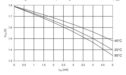
Figure 30-272. ATmega3290 A: I/O Pin Output Voltage vs. Sink Current, Ports A, C, D, E, F, G  $(V_{CC} = 5V)$
