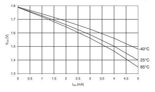
Figure 30-332. ATmega3290 PA: I/O Pin Output Voltage vs. Sink Current, Ports A, C, D, E, F, G  $(V_{CC}=5V)$
