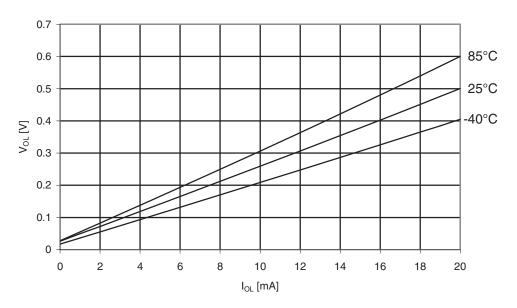
Figure 30-156.ATmega329A: I/O Pin Output Voltage vs. Sink Current, Port B (V<sub>CC</sub> = 2.7V)
