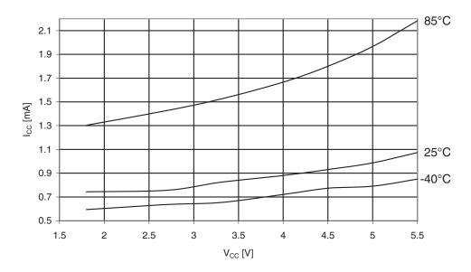
**Figure 30-139.** ATmega329A: Standby Supply Current vs.  $V_{CC}$  (Xtall and Resonator, Watchdog Timer Disabled)
