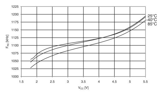
Figure 30-170. ATmega329A: Watchdog Oscillator Frequency vs. Temperature
