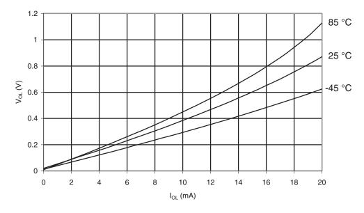
Figure 30-520. ATmega6490 A: I/O Pin Output Voltage vs. Sink Current, Port B ( $V_{CC} = 1.8V$ )
