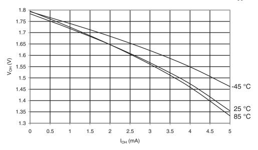
Figure 30-515. ATmega6490 A: I/O Pin Output Voltage vs. Sink Current, Ports A, C, D, E, F, G  $(V_{CC} = 5V)$
