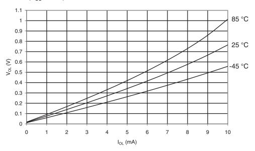
Figure 30-30. ATmega169A: I/O Pin Output Voltage vs. Sink Current, Ports A, C, D, E, F, G  $(V_{CC} = 1.8V)$
