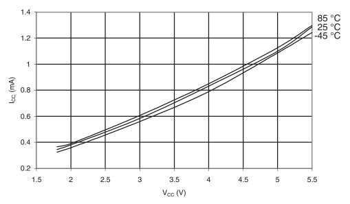
Figure 30-557.ATmega6490P: Idle Supply Current vs. V<sub>CC</sub> (32kHz Watch Crystal)
