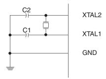
The Oscillator can operate in three different modes, each optimized for a specific frequency range. The operating mode is selected by the fuses CKSEL3...1 as shown in Table 9-5.
