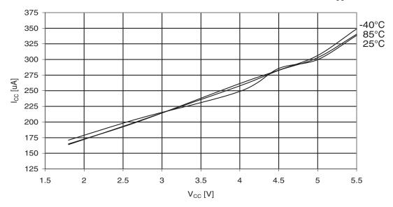
Figure 30-358.ATmega3290PA: AREF External Reference Current vs. V<sub>CC</sub>
