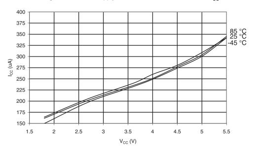
Figure 30-54. ATmega169A: Active Supply Current with ADC at 200kHz vs. V<sub>CC</sub>
