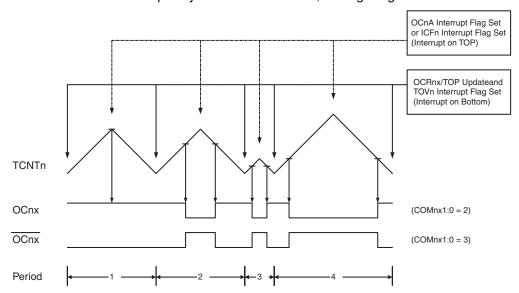
The Timer/Counter Overflow Flag (TOV1) is set at the same timer clock cycle as the OCR1x Registers are updated with the double buffer value (at BOTTOM). When either OCR1A or ICR1 is used for defining the TOP value, the OC1A or ICF1 Flag set when TCNT1 has reached TOP. The Interrupt Flags can then be used to generate an interrupt each time the counter reaches the TOP or BOTTOM value.
