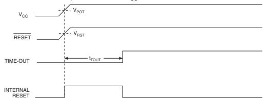
Figure 11-3. MCU Start-up, RESET Extended Externally
