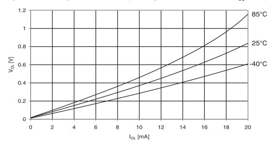
Figure 30-277.ATmega3290A: I/O Pin Output Voltage vs. Sink Current, Port B (V<sub>CC</sub> = 1.8V)
