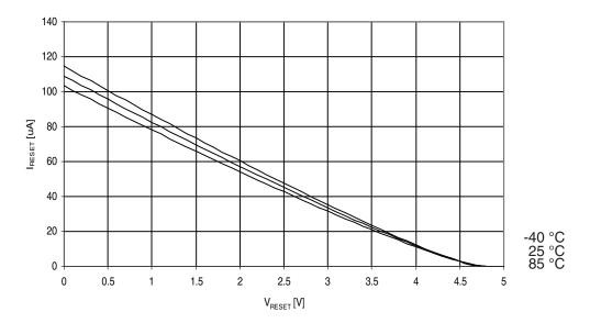
Figure 30-144. ATmega329A: Reset Pull-up Resistor Current vs. Reset Pin Voltage ( $V_{CC} = 2.7V$ )
