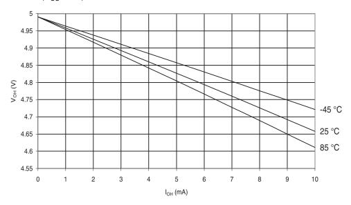
Figure 30-449. ATmega649P: I/O Pin Output Voltage vs. Source Current, Ports A, C, D, E, F, G  $(V_{CC}=2.7V)$
