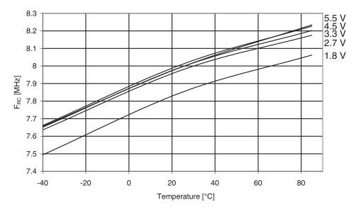
Figure 30-232.ATmega329PA: Calibrated 8MHz RC Oscillator Frequency vs. V<sub>CC</sub>
