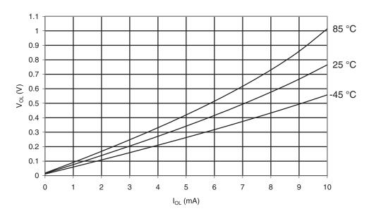
Figure 30-92. ATmega169PA: I/O Pin Output Voltage vs. Sink Current, Ports A, C, D, E, F, G  $(V_{CC}=1.8V)$
