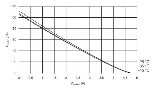
Figure 30-82. ATmega169PA: Reset Pull-up Resistor Current vs. Reset Pin Voltage (V<sub>CC</sub>=2.7V)
