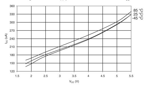
Figure 30-479. ATmega649P: Active Supply Current with ADC at 1MHz vs.  $V_{\rm CC}$
