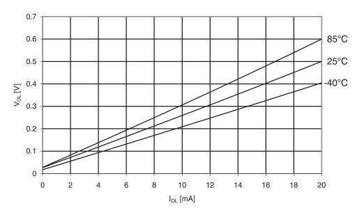
Figure 30-336.ATmega3290PA: I/O Pin Output Voltage vs. Sink Current, Port B (V<sub>CC</sub> = 2.7V)
