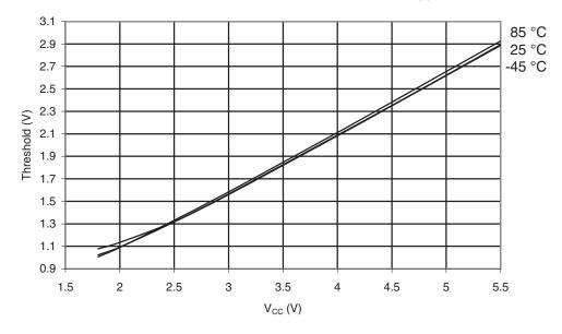
Figure 30-583. ATmega6490P: I/O Pin Input Threshold Voltage vs.  $V_{CC}$  ( $V_{IL}$ , I/O Pin Read as "0"
