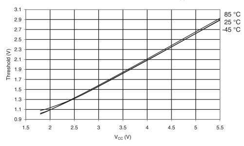
Figure 30-400. ATmega649A: I/O Pin Input Threshold Voltage vs.  $V_{CC}$  ( $V_{IL}$ , I/O Pin Read as "0")
