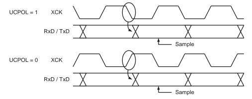
The UCPOLn bit UCRSC selects which XCK clock edge is used for data sampling and which is used for data change. As Figure 20-3 shows, when UCPOLn is zero the data will be changed at rising XCK edge and sampled at falling XCK edge. If UCPOLn is set, the data will be changed at falling XCK edge and sampled at rising XCK edge.
