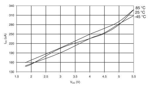
Figure 30-419.ATmega649A: AREF External Reference Current vs. V<sub>CC</sub>
