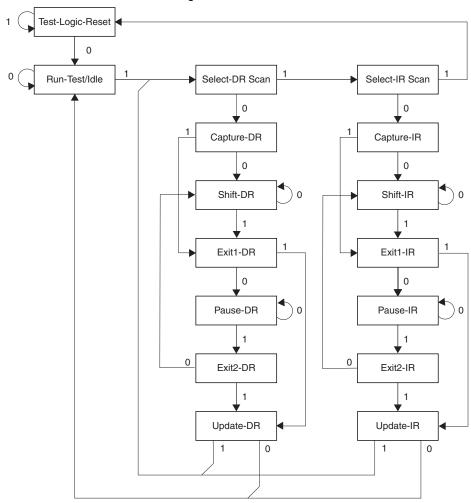
Figure 25-2. TAP Controller State Diagram
