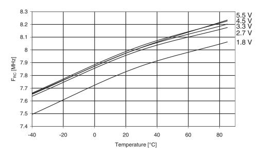
Figure 30-172. ATmega329A: Calibrated 8MHz RC Oscillator Frequency vs. V<sub>CC</sub>
