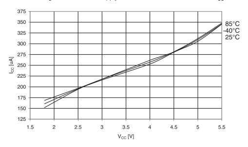
Figure 30-237. ATmega329PA: Active Supply Current with ADC at 1MHz vs.  $V_{\rm CC}$
