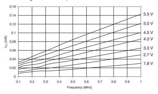
**Figure 30-607.**ATmega6490P: Reset Supply Current vs. V<sub>CC</sub> (1 - 20MHz, Excluding Current Through The Reset Pull-up)
