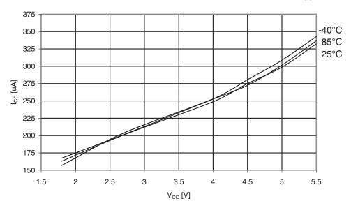
Figure 30-296. ATmega3290A: Active Supply Current with ADC at 200kHz vs.  $V_{CC}$
