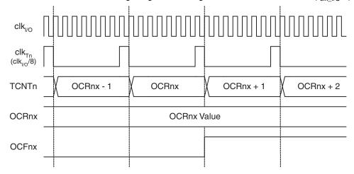
Figure 16-12 shows the count sequence close to TOP in various modes. When using phase and frequency correct PWM mode the OCR1x Register is updated at BOTTOM. The timing diagrams will be the same, but TOP should be replaced by BOTTOM, TOP-1 by BOTTOM+1 and so on. The same renaming applies for modes that set the TOV1 Flag at BOTTOM.
