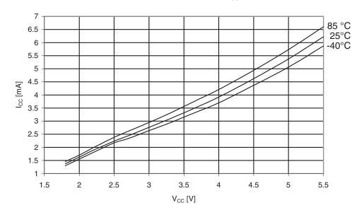
Figure 30-248.ATmega3290A: Active Supply Current vs. V<sub>CC</sub> (Internal RC Oscillator, 1MHz)
