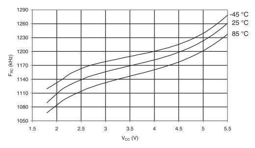
Figure 30-411. ATmega649A: Watchdog Oscillator Frequency vs. Temperature
