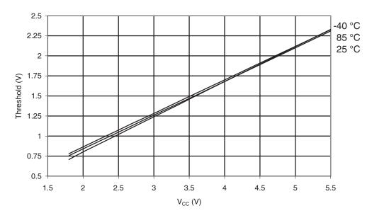
Figure 30-343. ATmega3290 PA: Reset Input Pin Hysteresis vs.  $V_{\rm CC}$
