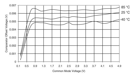
Figure 30-46. ATmega169A: Analog Comparator Offset Voltage vs. Common Mode Voltage  $(V_{CC} = 2.7V)$
