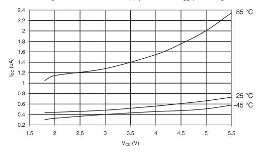
Figure 30-498.ATmega6490A: Power-down Supply Current vs. V<sub>CC</sub> (Watchdog Timer Enabled)
