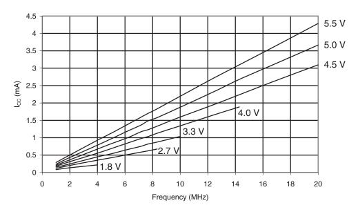
**Figure 30-494.** ATmega6490A: Idle Supply Current vs.  $V_{CC}$  (Internal RC Oscillator, 8MHz)
