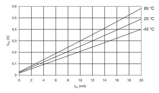
Figure 30-94. ATmega169PA: I/O Pin Output Voltage vs. Sink Current, Port B ( $V_{CC} = 2.7V$ )
