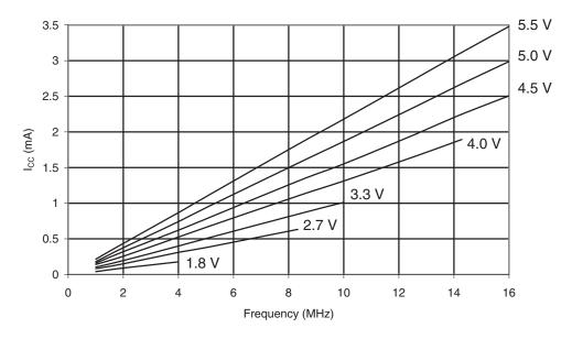
Figure 30-70. ATmega169PA: Idle Supply Current vs.  $V_{CC}$  (Internal RC Oscillator, 8MHz)
