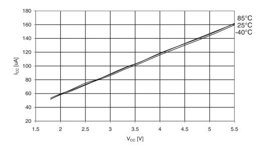
Figure 30-239.ATmega329PA: Watchdog Timer Current vs. V<sub>CC</sub>
