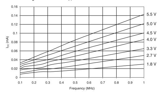
**Figure 30-485.**ATmega649P: Reset Supply Current vs. V<sub>CC</sub> (1 - 20MHz, Excluding Current Through The Reset Pull-up)
