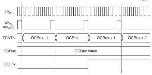
Figure 18-11 on page 158 shows the setting of OCF2A and the clearing of TCNT2 in CTC mode.
