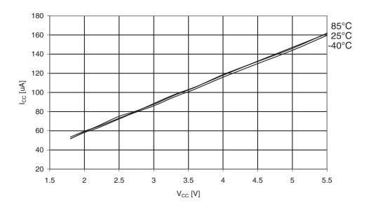
Figure 30-359. ATmega3290 PA: Watchdog Timer Current vs.  $V_{\rm CC}$
