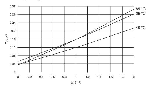
Figure 30-579.ATmega6490P: I/O Pin Output Voltage vs. Sink Current, Port B (V<sub>CC</sub> = 5V)
