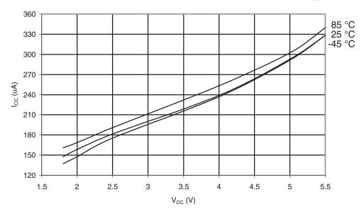
Figure 30-418. ATmega649A: Active Supply Current with ADC at 1MHz vs.  $V_{\rm CC}$
