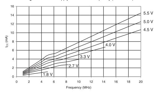
Figure 30-555. ATmega6490P: Idle Supply Current vs.  $V_{CC}$  (Internal RC Oscillator, 8MHz)
