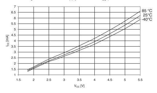
Figure 30-308.ATmega3290PA: Active Supply Current vs. V<sub>CC</sub> (Internal RC Oscillator, 1MHz)
