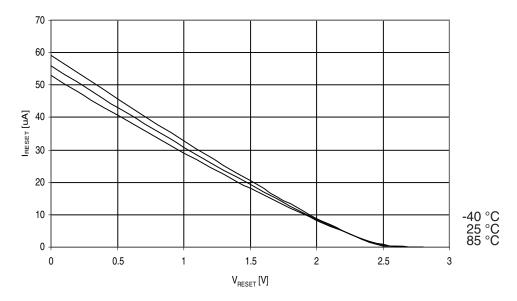
Figure 30-205. ATmega329PA: Reset Pull-up Resistor Current vs. Reset Pin Voltage ( $V_{CC} = 1.8V$ )
