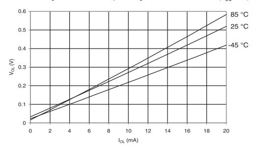
Figure 30-519.ATmega6490A: I/O Pin Output Voltage vs. Sink Current, Port B (V<sub>CC</sub> = 2.7V)
