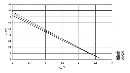
Figure 30-202. ATmega329PA: I/O Pin Pull-up Resistor Current vs. Input Voltage (V<sub>CC</sub> = 1.8V)
