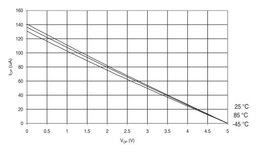
Figure 30-443. ATmega649P: I/O Pin Pull-up Resistor Current vs. Input Voltage (V<sub>CC</sub> = 2.7V)
