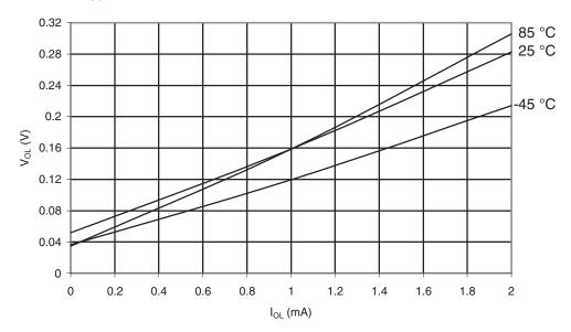
Figure 30-457. ATmega649P: I/O Pin Output Voltage vs. Sink Current, Port B ( $V_{CC} = 5V$ )
