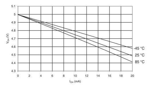
Figure 30-88. ATmega169PA: I/O Pin Output Voltage vs. Source Current, Port B (V<sub>CC</sub> = 2.7V)
