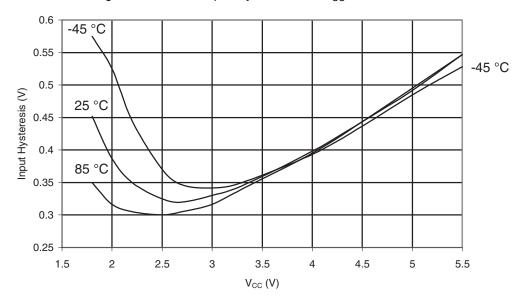
Figure 30-402. ATmega649A: Reset Input Threshold Voltage vs. V<sub>CC</sub> (V<sub>IH</sub>, Reset Pin Read as "1")
