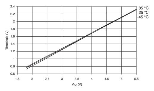
Figure 30-39. ATmega169A: Reset Input Pin Hysteresis vs. V<sub>CC</sub>
