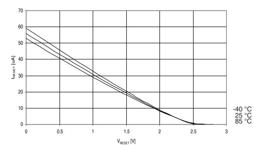
**Figure 30-325.** ATmega3290PA: Reset Pull-up Resistor Current vs. Reset Pin Voltage  $(V_{CC}=1.8V)$
