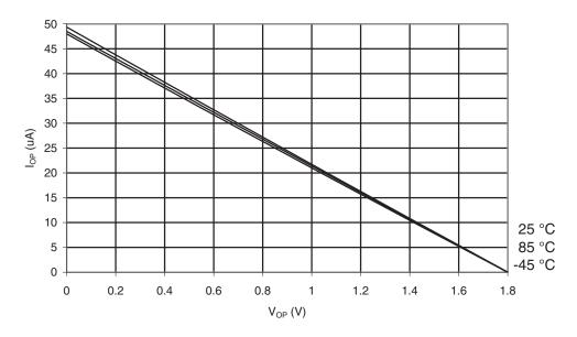
Figure 30-19. ATmega169A: Reset Pull-up Resistor Current vs. Reset Pin Voltage (V<sub>CC</sub> = 5V)
