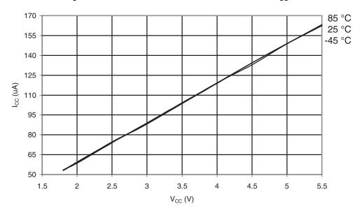
Figure 30-542.ATmega6490A: Watchdog Timer Current vs. V<sub>CC</sub>
