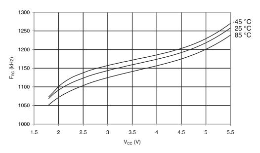
Figure 30-110. ATmega169PA: Watchdog Oscillator Frequency vs. Temperature
