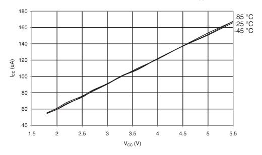
Figure 30-57. ATmega169A: Watchdog Timer Current vs.  $V_{CC}$
