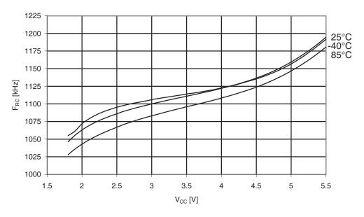
Figure 30-290. ATmega3290A: Watchdog Oscillator Frequency vs. Temperature
