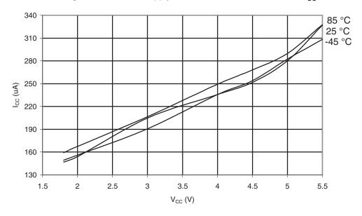
Figure 30-602. ATmega6490P: AREF External Reference Current vs.  $V_{CC}$
