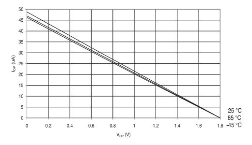
Figure 30-567. ATmega649A: Reset Pull-up Resistor Current vs. Reset Pin Voltage (V<sub>CC</sub> = 5V)
