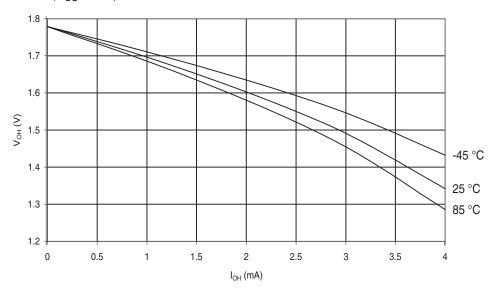
Figure 30-573.ATmega6490P: I/O Pin Output Voltage vs. Source Current, Port B (V<sub>CC</sub>= 5V)
