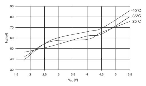
Figure 30-181. ATmega329A: Programming Current vs. V<sub>CC</sub>
