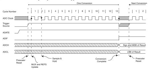
Figure 23-7. ADC Timing Diagram, Free Running Conversion
