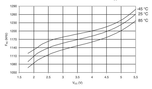
Figure 30-594. ATmega6490P: Watchdog Oscillator Frequency vs. Temperature
