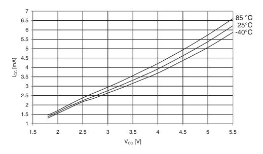
Figure 30-188.ATmega329PA: Active Supply Current vs. V<sub>CC</sub> (Internal RC Oscillator, 1MHz)
