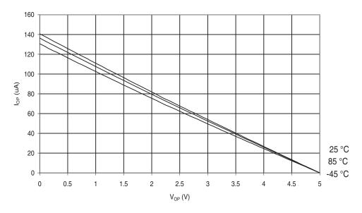
Figure 30-382.ATmega649A: I/O Pin Pull-up Resistor Current vs. Input Voltage (V<sub>CC</sub> = 2.7V)
