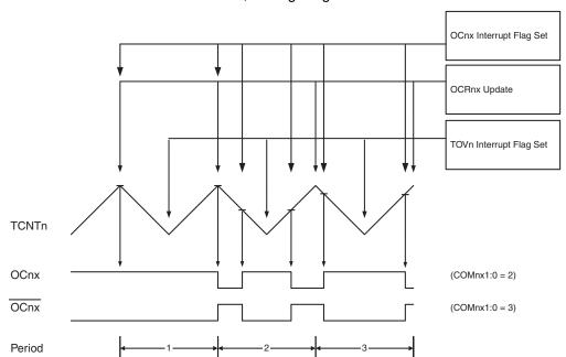
Figure 18-7. Phase Correct PWM Mode, Timing Diagram
