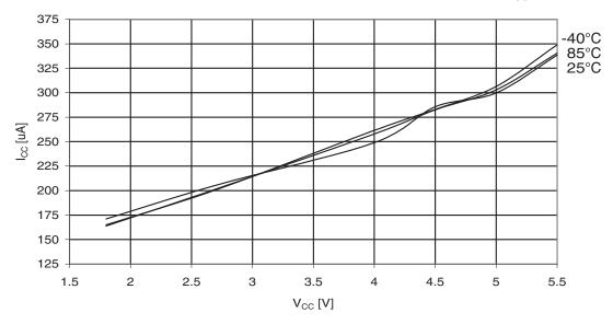
Figure 30-298. ATmega3290A: AREF External Reference Current vs.  $V_{CC}$
