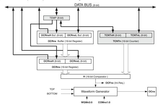
Figure 16-4. Output Compare Unit, Block Diagram
