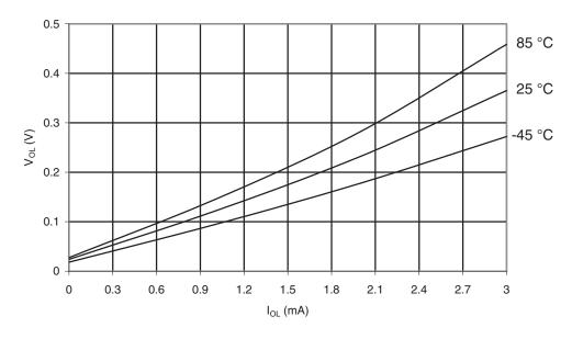
Figure 30-93. ATmega169PA: I/O Pin Output Voltage vs. Sink Current, Port B ( $V_{CC} = 5V$ )
