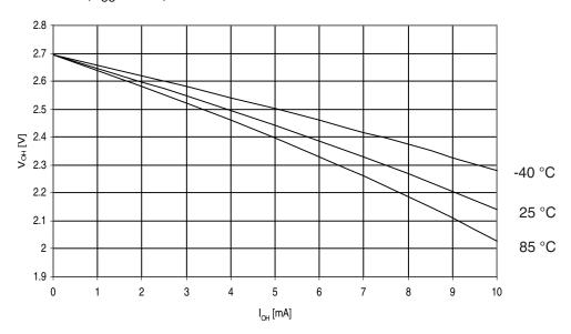
Figure 30-208. ATmega329 PA: I/O Pin Output Voltage vs. Source Current, Ports A, C, D, E, F, G ( $V_{CC} = 1.8V$ )
