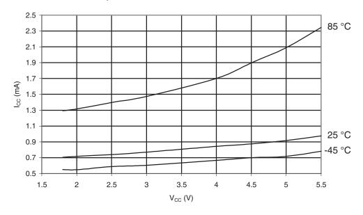
**Figure 30-441.**ATmega649P: Standby Supply Current vs. V<sub>CC</sub> (Xtall and Resonator, Watchdog Timer Disabled)
