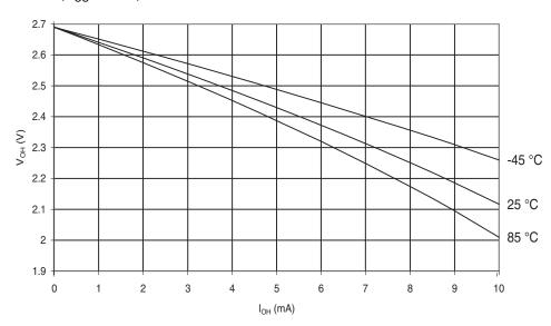
Figure 30-511. ATmega6490A: I/O Pin Output Voltage vs. Source Current, Ports A, C, D, E, F, G  $(V_{CC} = 1.8V)$
