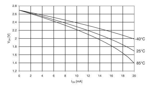
Figure 30-151.ATmega329A: I/O Pin Output Voltage vs. Source Current, Port B (V<sub>CC</sub> = 1.8V)
