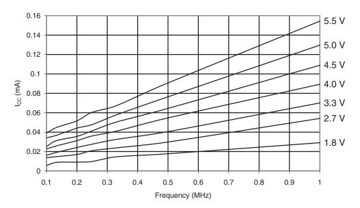
**Figure 30-61.** ATmega169A: Reset Supply Current vs. V<sub>CC</sub> (1 - 16MHz, Excluding Current Through The Reset Pull-up)
