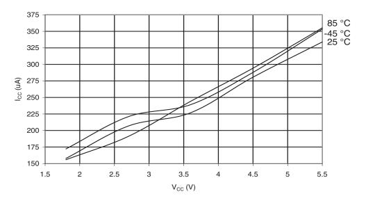
Figure 30-55. ATmega169A: Active Supply Current with ADC at 1MHz vs.  $V_{\rm CC}$
