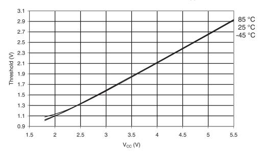
Figure 30-35. ATmega169A: I/O Pin Input Threshold Voltage vs.  $V_{CC}$  ( $V_{IL}$ , I/O Pin Read as "0"
