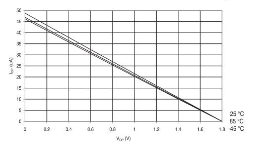
Figure 30-384. ATmega649A: Reset Pull-up Resistor Current vs. Reset Pin Voltage (V<sub>CC</sub> = 5V)
