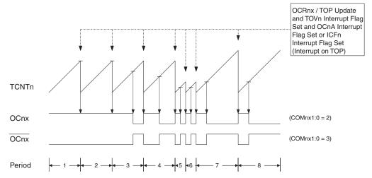
The Timer/Counter Overflow Flag (TOV1) is set each time the counter reaches TOP. In addition the OC1A or ICF1 Flag is set at the same timer clock cycle as TOV1 is set when either OCR1A or ICR1 is used for defining the TOP value. If one of the interrupts are enabled, the interrupt handler routine can be used for updating the TOP and compare values.
