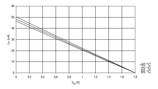
Figure 30-323. ATmega3290PA: Reset Pull-up Resistor Current vs. Reset Pin Voltage (V<sub>CC</sub>=5V)
