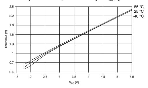
Figure 30-280. ATmega3290 A: I/O Pin Input Hysteresis vs.  $V_{CC}$
