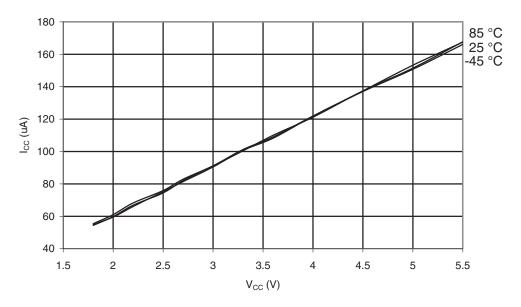
Figure 30-119.ATmega169PA: Watchdog Timer Current vs. V<sub>CC</sub>
