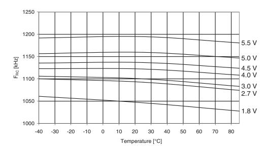
Figure 30-351.ATmega3290PA: Calibrated 8MHz RC Oscillator Frequency vs. Temperature
