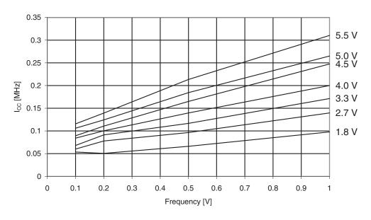
Figure 30-251.ATmega3290A: Idle Supply Current vs. Frequency (1 - 20MHz)
