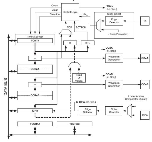
Figure 16-1. 16-bit Timer/Counter Block Diagram<sup>(1)</sup>
