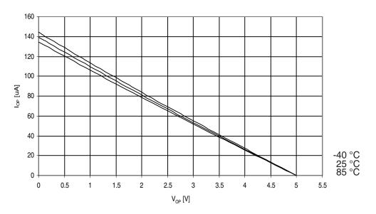
Figure 30-261. ATmega3290 A: I/O Pin Pull-up Resistor Current vs. Input Voltage ( $V_{CC} = 2.7V$ )
