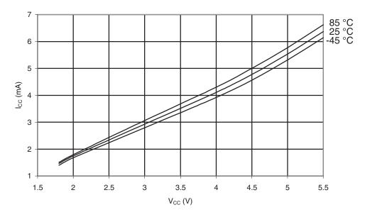
Figure 30-368.ATmega649A: Active Supply Current vs. V<sub>CC</sub> (Internal RC Oscillator, 1MHz)
