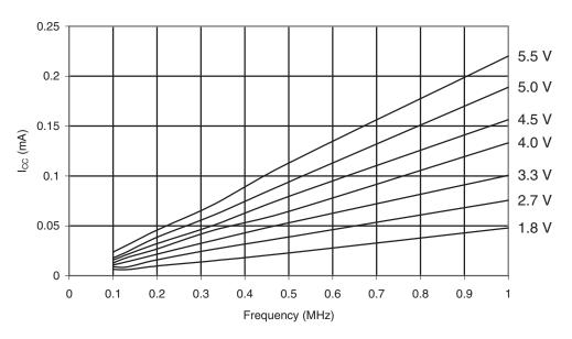
Figure 30-69. ATmega169PA: Idle Supply Current vs. Frequency (1 - 16MHz)
