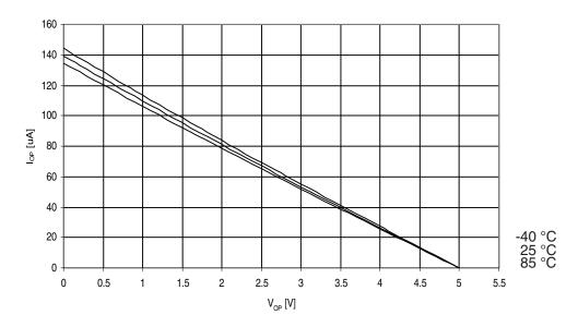
Figure 30-321.ATmega3290PA: I/O Pin Pull-up Resistor Current vs. Input Voltage (V<sub>CC</sub> = 2.7V)
