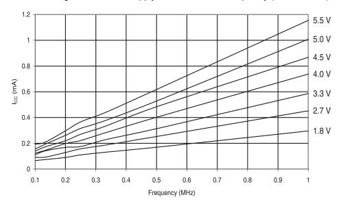
Figure 30-427.ATmega649P: Active Supply Current vs. Frequency (1 - 20MHz)
