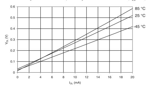
Figure 30-580.ATmega6490P: I/O Pin Output Voltage vs. Sink Current, Port B (V<sub>CC</sub> = 2.7V)
