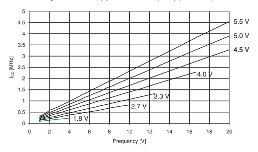
Figure 30-132. ATmega329A: Idle Supply Current vs.  $V_{CC}$  (Internal RC Oscillator, 8MHz)
