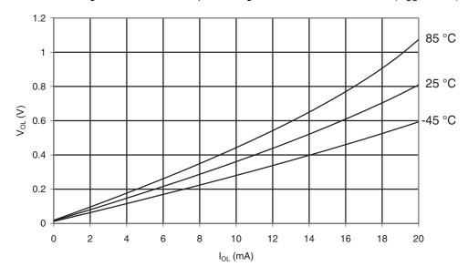
Figure 30-33. ATmega169A: I/O Pin Output Voltage vs. Sink Current, Port B (V<sub>CC</sub> = 1.8V)
