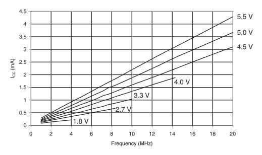
Figure 30-433. ATmega649P: Idle Supply Current vs.  $V_{CC}$  (Internal RC Oscillator, 8MHz)
