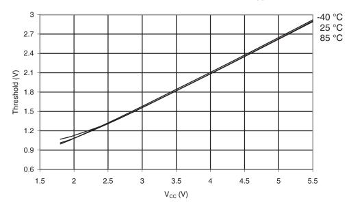
Figure 30-159. ATmega329A. I/O Pin Input Threshold Voltage vs.  $V_{CC}$  ( $V_{IL}$ , I/O Pin Read as "0")
