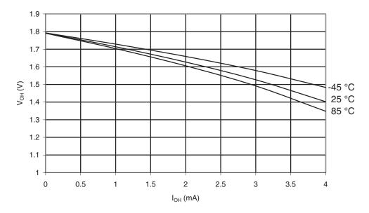
Figure 30-87. ATmega169PA: I/O Pin Output Voltage vs. Source Current, Port B (V<sub>CC</sub>= 5V)
