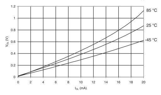
Figure 30-398. ATmega649A: I/O Pin Output Voltage vs. Sink Current, Port B ( $V_{CC} = 1.8V$ )
