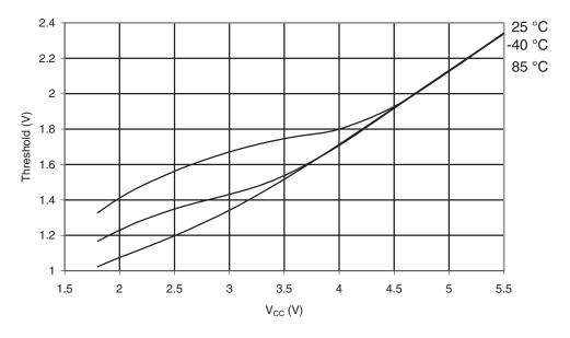
Figure 30-162.ATmega329A: Reset Input Threshold Voltage vs. V<sub>CC</sub> (V<sub>IL</sub>,Reset Pin Read as "0")
