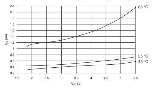
$\textbf{Figure 30-376.} \\ \textbf{ATmega649A: Power-down Supply Current vs. } \\ \textbf{V}_{\textit{CC}} \ (\textbf{Watchdog Timer Enabled})$
