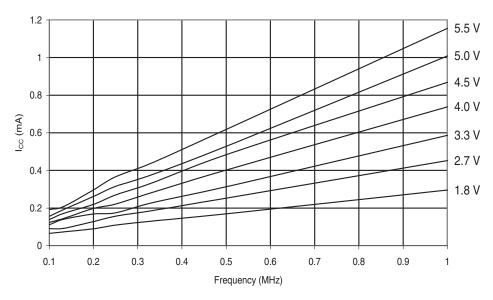
Figure 30-488. ATmega6490A: Active Supply Current vs. Frequency (1 - 20MHz)
