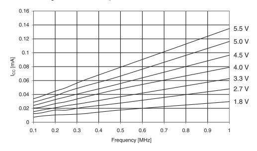
**Figure 30-363.**ATmega3290PA: Reset Supply Current vs. V<sub>CC</sub> (1 - 20MHz, Excluding Current Through The Reset Pull-up)
