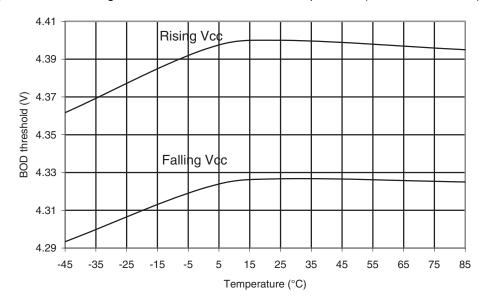
Figure 30-406.ATmega649A: BOD Thresholds vs. Temperature (BOD Level is 2.7V)
