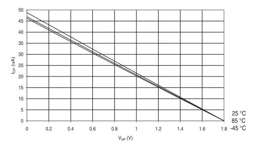
Figure 30-445.ATmega649P: Reset Pull-up Resistor Current vs. Reset Pin Voltage (V<sub>CC</sub> = 5V)
