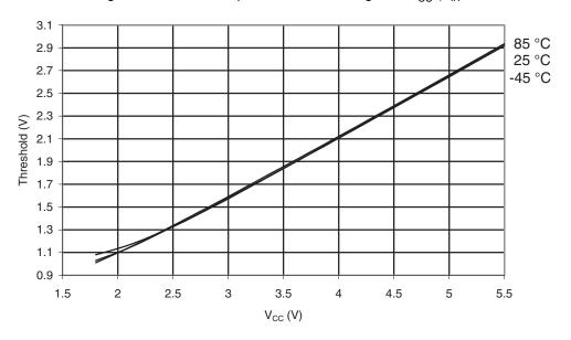
Figure 30-97. ATmega169PA. I/O Pin Input Threshold Voltage vs.  $V_{CC}$  ( $V_{IL}$ , I/O Pin Read as "0"
