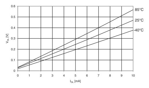
Figure 30-213. ATmega329 PA. I/O Pin Output Voltage vs. Sink Current, Ports A, C, D, E, F, G  $(V_{CC}=2.7V)$
