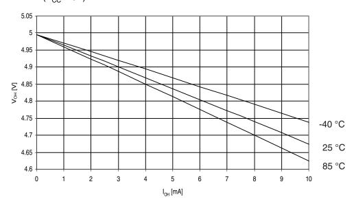
Figure 30-267. ATmega3290 A: I/O Pin Output Voltage vs. Source Current, Ports A, C, D, E, F, G  $(V_{CC} = 2.7V)$
