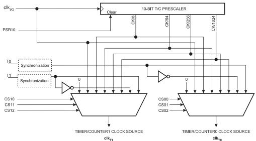
Figure 17-2. Prescaler for Timer/Counter0 and Timer/Counter1<sup>(1)</sup>
