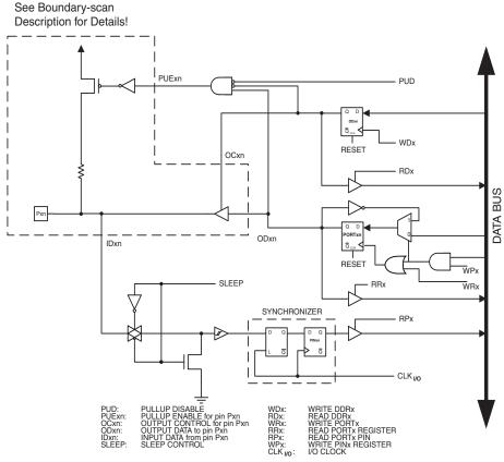
Figure 26-3. General Port Pin Schematic Diagram
