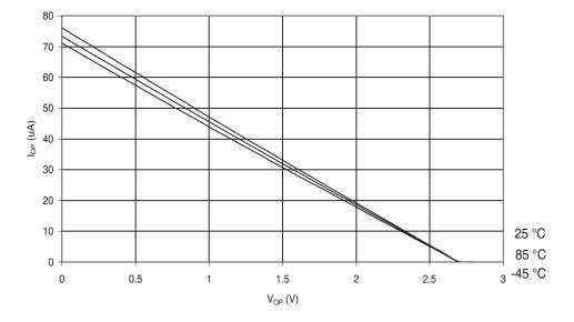
Figure 30-566.ATmega6490P: I/O Pin Pull-up Resistor Current vs. Input Voltage (V<sub>CC</sub> = 1.8V)
