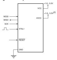
Notes: 1. If the device is clocked by the internal Oscillator, it is no need to connect a clock source to the XTAL1 pin.
