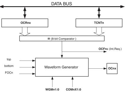
The OCR2A Register is double buffered when using any of the Pulse Width Modulation (PWM) modes. For the Normal and Clear Timer on Compare (CTC) modes of operation, the double buffering is disabled. The double buffering synchronizes the update of the OCR2A Compare Register to either top or bottom of the counting sequence. The synchronization prevents the occurrence of odd-length, non-symmetrical PWM pulses, thereby making the output glitch-free.
