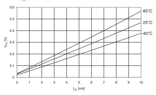
Figure 30-273. ATmega3290 A. I/O Pin Output Voltage vs. Sink Current, Ports A, C, D, E, F, G  $(V_{CC}=2.7V)$
