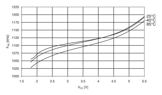
Figure 30-350.ATmega3290PA: Watchdog Oscillator Frequency vs. Temperature
