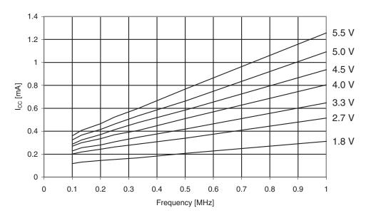
Figure 30-186.ATmega329PA: Active Supply Current vs. Frequency (1 - 20MHz)
