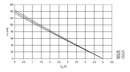
Figure 30-141. ATmega329A: I/O Pin Pull-up Resistor Current vs. Input Voltage (V<sub>CC</sub> = 2.7V)
