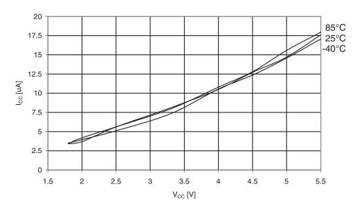
Figure 30-300. ATmega3290 A: Analog Comparator Current vs.  $V_{\rm CC}$
