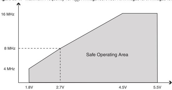
**Figure 29-2.** Maximum Frequency vs. V<sub>CC</sub> (0 - 20MHz) ATmega329A/ATmega329PA/ATmega3290A/ATmega3290PA/ATmega6490A/ ATmega6490P
