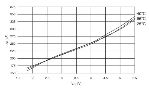
Figure 30-176.ATmega329A: Active Supply Current with ADC at 200kHz vs. V<sub>CC</sub>
