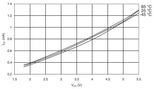
Figure 30-496.ATmega6490A: Idle Supply Current vs. V<sub>CC</sub> (32kHz Watch Crystal)
