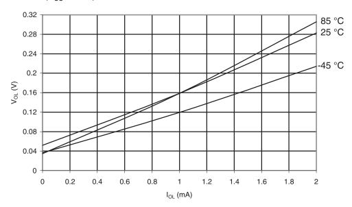
Figure 30-396. ATmega649A: I/O Pin Output Voltage vs. Sink Current, Port B ( $V_{CC} = 5V$ )
