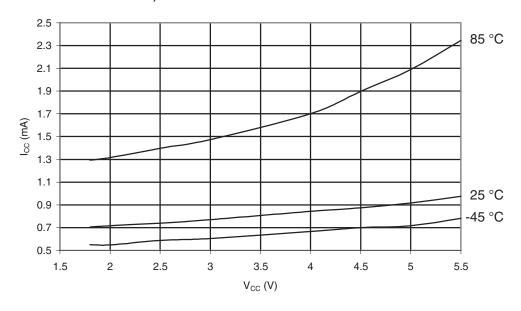
**Figure 30-380.** ATmega649A: Standby Supply Current vs.  $V_{CC}$  (Xtall and Resonator, Watchdog Timer Disabled)
