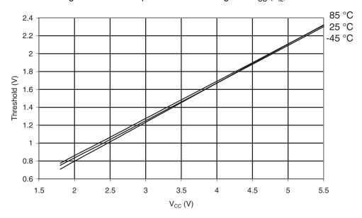
Figure 30-465.ATmega649P: Reset Input Pin Hysteresis vs. V<sub>CC</sub>
