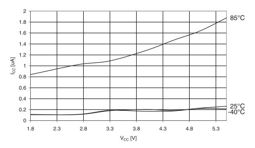
Figure 30-316.ATmega3290PA: Power-down Supply Current vs. V<sub>CC</sub> (Watchdog Timer Enabled)
