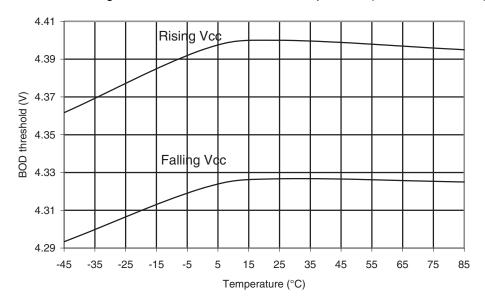
Figure 30-589.ATmega6490P: BOD Thresholds vs. Temperature (BOD Level is 2.7V)
