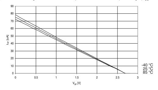
Figure 30-262. ATmega3290A: I/O Pin Pull-up Resistor Current vs. Input Voltage ( $V_{CC} = 1.8V$ )
