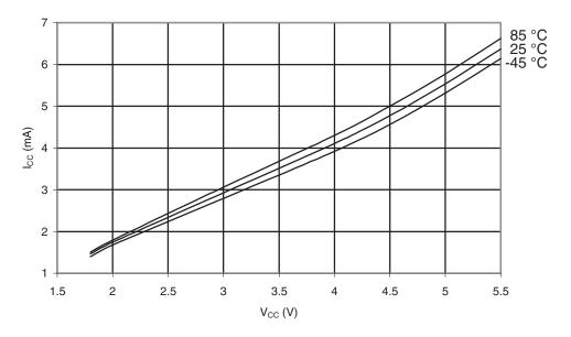
Figure 30-551.ATmega6490P: Active Supply Current vs. V<sub>CC</sub> (Internal RC Oscillator, 1MHz)
