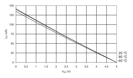
Figure 30-79. ATmega169PA: I/O Pin Pull-up Resistor Current vs. Input Voltage (V<sub>CC</sub> = 2.7V)
