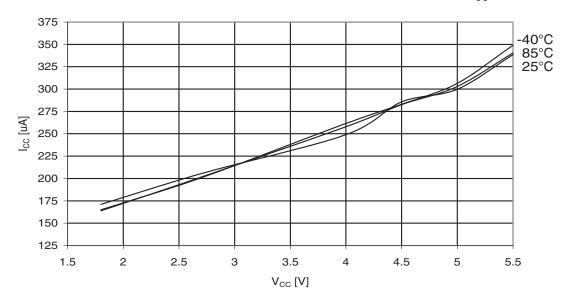
Figure 30-238.ATmega329PA: AREF External Reference Current vs. V<sub>CC</sub>
