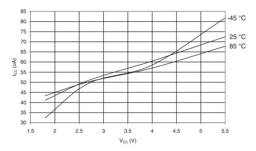
Figure 30-59. ATmega169A: Programming Current vs. V<sub>CC</sub>
