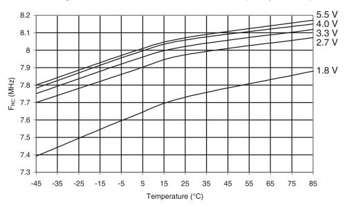
Figure 30-474.ATmega649P: Calibrated 8MHz RC Oscillator Frequency vs. V<sub>CC</sub>
