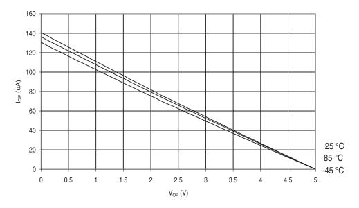
Figure 30-565.ATmega6490P: I/O Pin Pull-up Resistor Current vs. Input Voltage (V<sub>CC</sub> = 2.7V)
