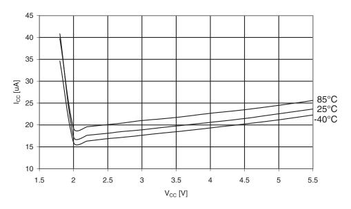
Figure 30-235.ATmega329PA: Active Supply Current with ADC at 50kHz vs. V<sub>CC</sub>
