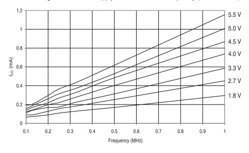
Figure 30-366.ATmega649A: Active Supply Current vs. Frequency (1 - 20MHz)
