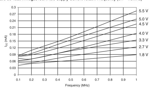
Figure 30-493. ATmega6490A: Idle Supply Current vs. Frequency (1 - 20MHz)
