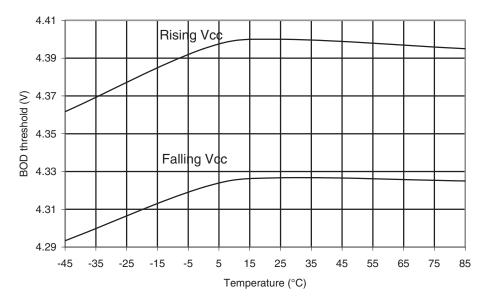
Figure 30-528.ATmega6490A: BOD Thresholds vs. Temperature (BOD Level is 2.7V)
