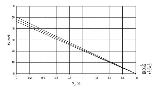
Figure 30-203. ATmega329PA: Reset Pull-up Resistor Current vs. Reset Pin Voltage (V<sub>CC</sub> = 5V)
