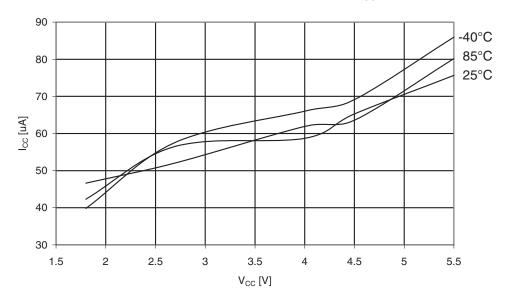
Figure 30-361.ATmega3290PA: Programming Current vs. V<sub>CC</sub>
