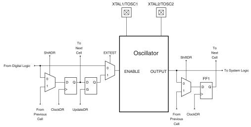
Table 26-2 summaries the scan registers for the external clock pin XTAL1, oscillators with XTAL1/XTAL2 connections as well as 32kHz Timer Oscillator.
