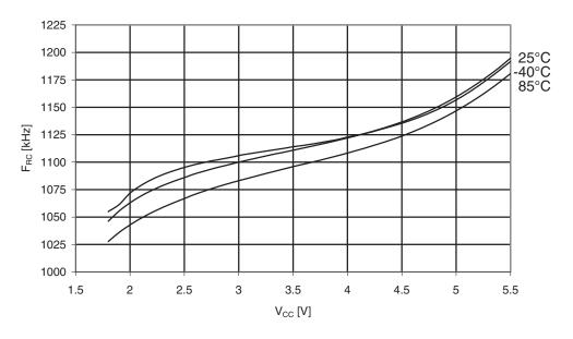
Figure 30-230. ATmega329PA: Watchdog Oscillator Frequency vs. Temperature
