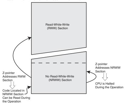
Figure 27-1. Read-While-Write vs. No Read-While-Write
