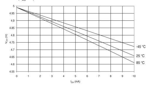
**Figure 30-571.** ATmega6490P: I/O Pin Output Voltage vs. Source Current, Ports A, C, D, E, F, G  $(V_{CC}=2.7V)$
