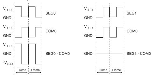
Figure 24-3. Driving a LCD with One Common Terminal
