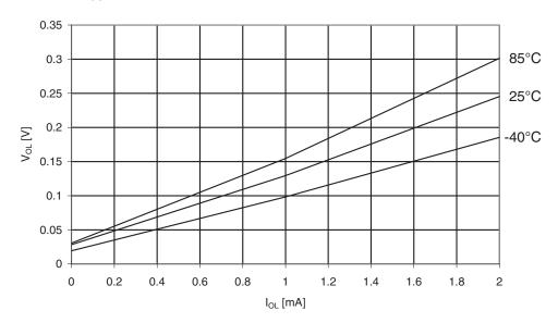
Figure 30-215.ATmega329PA: I/O Pin Output Voltage vs. Sink Current, Port B (V<sub>CC</sub> = 5V)
