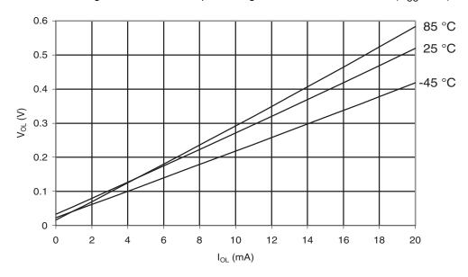
Figure 30-458.ATmega649P: I/O Pin Output Voltage vs. Sink Current, Port B (V<sub>CC</sub> = 2.7V)
