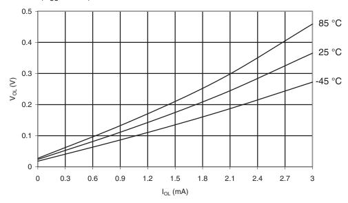
Figure 30-31. ATmega169A: I/O Pin Output Voltage vs. Sink Current, Port B ( $V_{CC} = 5V$ )
