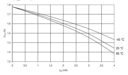
Figure 30-512. ATmega6490 A: I/O Pin Output Voltage vs. Source Current, Port B ( $V_{CC}$ = 5V)
