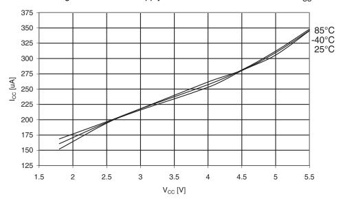
Figure 30-297.ATmega3290A: Active Supply Current with ADC at 1MHz vs. V<sub>CC</sub>
