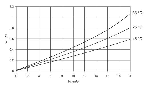
Figure 30-95. ATmega169PA: I/O Pin Output Voltage vs. Sink Current, Port B (V<sub>CC</sub> = 1.8V)
