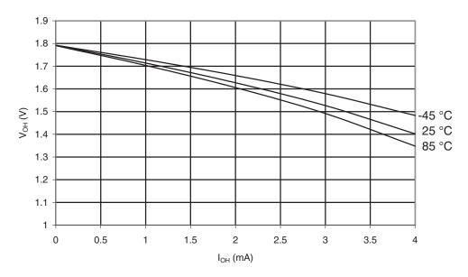
Figure 30-25. ATmega169A: I/O Pin Output Voltage vs. Source Current, Port B (V<sub>CC</sub>= 5V)
