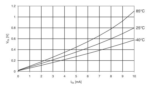
Figure 30-274. ATmega3290 A: I/O Pin Output Voltage vs. Sink Current, Ports A, C, D, E, F, G  $(V_{CC}=1.8V)$
