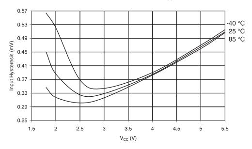
Figure 30-221. ATmega329PA: Reset Input Threshold Voltage vs.  $V_{CC}$  ( $V_{IH}$ , Reset Pin Read as "1")
