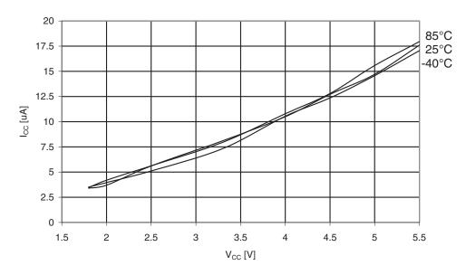
Figure 30-180.ATmega329A: Analog Comparator Current vs. V<sub>CC</sub>
