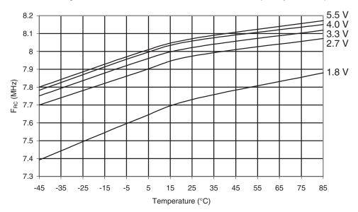
Figure 30-596.ATmega6490P: Calibrated 8MHz RC Oscillator Frequency vs. V<sub>CC</sub>
