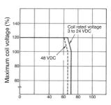
Ambient temperature (°) Note: The maximum coil voltage refers to the maximum value in a varying range of operating power voltage, not a continuous voltage.
